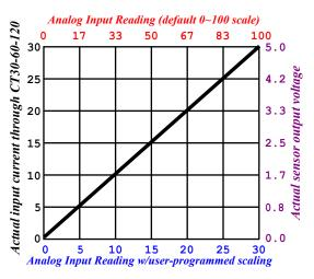
Note that these settings only affect the way the data is <u>displayed</u> – the data samples themselves are always stored in the unit's memory as a 10-bit binary number representing the inputs' 0~5V input range, and are only converted to the scale range you've set when the readings are displayed on-screen or downloaded from the **Logging** page. This means that if you change the scale on an Analog-Input channel, and then subsequently
