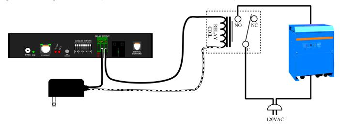
Note: ITWatchDogs <u>strongly</u> recommends consulting a qualified and licensed electrician to set up this kind of secondary-relay control method, as hazardous voltages may be present when attempting to connect equipment directly to AC line voltages. Also, a licensed electrician will be more familiar with any local building codes which might dictate the type of wiring and contactors that must be used, and how they must be installed.
