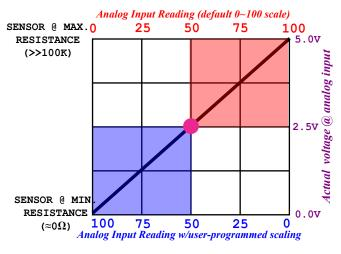
above, will result in a reading of "0"; once the surface under the sensor gets damp enough to allow current to flow between the contacts, the sensor's resistance will decrease (or, put another way, its conductivity will increase), allowing the input voltage to drop towards 0V and causing the scaled value to increase towards "100". Once the sensor is wet enough to cause the input voltage to fall below the halfway mark of +2.5V, the alarm will trip, as shown in the blue-shaded area.
