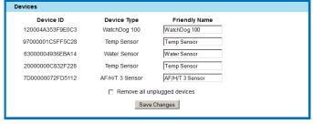
In the example shown here, there are four external sensors attached: two RT-series temperature sensors, an RTAFHD3 temperature / airflow / humidity "combo" sensor, and a CCAT analog-to-digital converter programmed for use with a water sensor such as the ITWatchDogs WD-1 kit.
