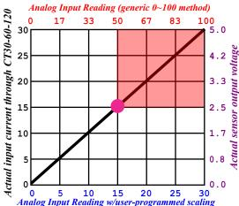
The graph at left illustrates this action. The spot in the center represents an alarm threshold which the user wishes to set so that the alarm trips when the reading goes above 15A. Using the default  $0\sim$
