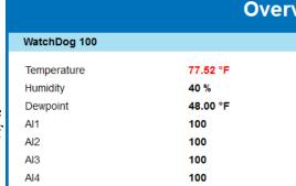
In addition, any sensor value(s) which have exceeded any of the alarm the shold(s) set on them will be displayed in **red text**, instead of the usual black text, as shown here.
