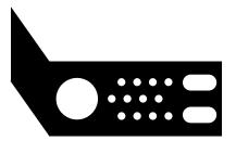
The WatchDog-100 also comes supplied with a pair of 1-U mounting brackets, to allow the unit to be mounted in a standard 19" rack-mount cabinet if desired. These will normally already be mounted to the unit when you first receive it, since they help keep the unit from moving around inside the box during shipment, but can be easily removed with a Philips-head screwdriver if you wish to mount the unit some other way.
