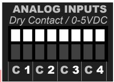
WARNING: Reversing the polarity of the wires on such sensors will result in incorrect sensor behavior, and may damage the sensor and/or the WatchDog-100 itself!
