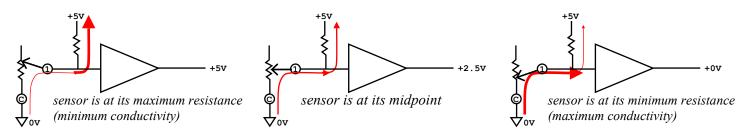
On the right, the sensor is at its minimum resistance, pulling the analog-input channel down to 0V; the channel will be seen as having a 0V input signal.
