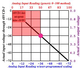
In this kind of application, however, it is important to note that when you set an alarm threshold to trip "above" or "below" a certain point, the WatchDog-100 looks at these numbers in strictly mathematical terms. If you wanted to set an alarm to trip once the battery voltage has fallen to –36VDC or less, as represented by the red-shaded area in the graph above, you would actually need to set the threshold to trip "above –36.0" since, mathematically speaking, –35 is greater than –36.
