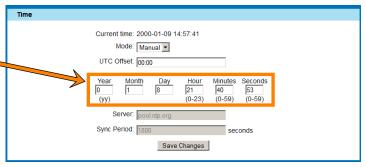
can either be on your internal network, or it can be a publicly-accessible NTP service such as ntp.pool.org. In this mode, the manual time-setting fields described above are greyed out and ignored. The **Server** field specifies the NTP time server to be used, while the **Sync Period** field determines how frequently the WatchDog-100 will poll the NTP service to keep the clock synchronized.
