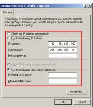
your browser returns an error page indicating that the address can't be found, go through the above steps again and double-check the network settings to make sure **IP address** and **Subnet Mask** are set correctly. Also note that the instructions above are assuming a direct connection, PC to WatchDog-100; if you have connected the WatchDog-100 to a network switch instead, it's possible that the addresses suggested above are in conflict with another device already on your network.)
