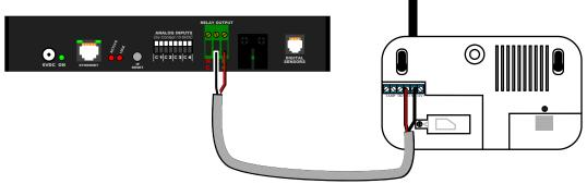
If an alarm threshold which has the relay selected as one of its actions is tripped, the relay will energize, closing the NO contact pair and activating the dialer.
