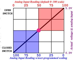
The graph above illustrates this action. The spot in the center represents an alarm threshold which is set so that the alarm trips when the reading goes above 50. With the default Min=0, Max=100 scaling, this would represents an actual input voltage at the analog-input terminal of +2.5V, and so the alarm would trip once the input voltage went higher than +2.5V and the scaled reading went above 50, as shown in the red-shaded area.
