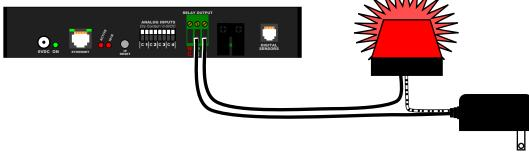
Notice how an external power supply is required to drive the strobe lamp. It is important to keep in mind, when choosing external devices, that the WatchDog-100's relay contacts do <u>not</u> provide power to drive external equipment directly; they are strictly an SPDT (Single-Pole-Double-Throw)
