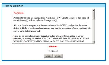
The default state is *Disabled*, meaning that the RPM-X2's relays can only be operated manually by the user from the *Control* tab, any settings related to automatic control will be grayed out or struck through, and any attempt to select the relays as alarm actions on the *Alarms* tab will be ignored. Clicking the acceptance checkbox and the *Enable* button will switch this feature to the *Enabled* state, allowing you to use the relays as alarm actions.
